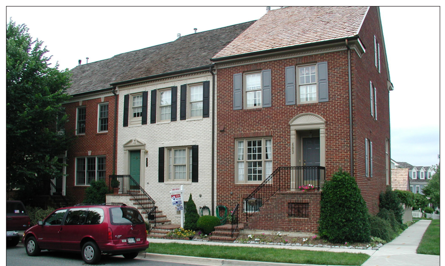
Rowhouses articulated as individual buildings with different materials and colors (facade differentiation).
