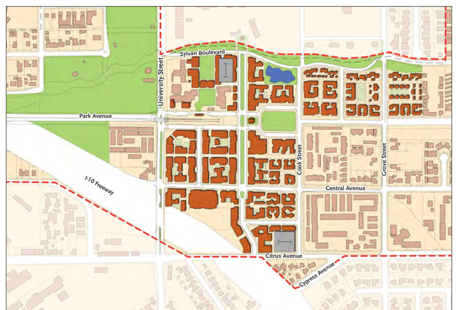
Illustrative Phase 5. The following are built: the road connecting the Rambla to Citrus Avenue and the westbound I-10 Cypress Avenue off-ramp; the park-once garage; the mixed-use and residential building to the south of Central Avenue.
